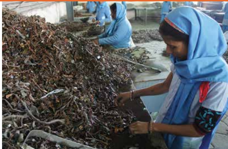
(At top) CMR executives P.M. Gautam, CEO, and Mohan Agarwal, managing director, visit the firm's Unit 1 facility in Palwal. At CMR, Zorba smaller than 35 mm is sized and then sent through a wash line (middle) for further sorting by density. A CMR employee (above) sorts copper and brass recovered from the sorting line.
